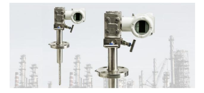
Accuracy: ± 1 % uncalibrated, ±0.5% calibrated w/ Tx Repeatability: ± 0.1% of rate Process temperature: Up to 1100 °F Pressure Rating: Up to 1500psi Minimum Reynolds Number: 50,000 Permanent Pressure Loss: 5% of DP Max Turn Down Ratio (TDR): Typical 10 to 1 Maximum Viscosity: 100 cP
