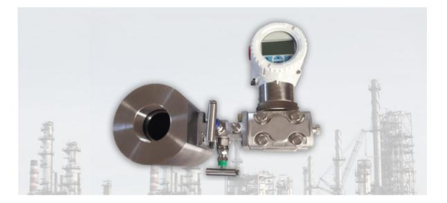
Accuracy: ± 2 % uncalibrated, ±0.50% calibrated w/ Tx Repeatability: ± 0.1% of rate Process temperature: Up to 1100 °F Pressure Rating: Up to 1500psi Minimum Reynolds Number: 500 Turn Down Ratio (TDR): Typical 10 to 1 Maximum Viscosity: Up to 5000 cP
